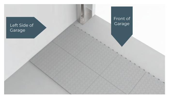
Leave a 0.5" inch gap between the wall and the tiles to allow for expansion due to temperature variations. If no space is left, the tiles will warp due to thermal expansion.
